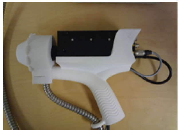
Fig. 2. Hand-held hyperspectral imager in holder. Ringlight is in front of the imager.
