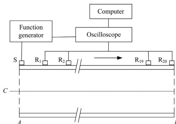
**Fig. 1.** Multi-channel acoustic set-up on a schematized open-cut pipe. S is source position.  $R_1$  to  $R_{20}$  are twenty receiver positions. A is the pipe's near end. B is the pipe's remote end. Line C is the axis of the pipe. Not to scale.
