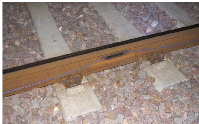
Fig. 1. FBG sensor installed on the rail neutral line to detect the temperature change.
