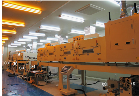
Fig. 1. Photo of R2R printing system considered in this study. (a) Unwinding, (b) infeeding, (c) 1st printing, (d) drying, (e) 2nd printing, (f) outfeeding, and (g) rewinding sections.
