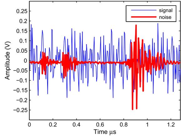
Fig. 2. Plot of typical signal (in blue) and noise (in red) for a SNR of 7 dB and for the duration of one typical OFDM symbol. Sampling rate was 200 MHz. (For interpretation of the references to color in this figure legend, the reader is referred to the web version of this article.)
