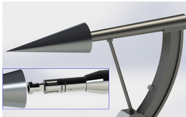
Fig. 1. The model-balance-sting system and its connection detail.
