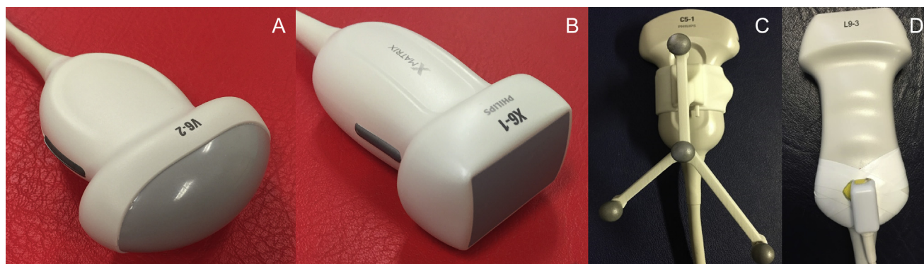
Figure 1. Three-dimensional ultrasound techniques. From left to right: (A) mechanical transducer; (B) matrix transducer; (C) standard curved transducer adapted for freehand scanning using optical tracking; (D) standard linear transducer adapted for freehand scanning using magnetic tracking.
