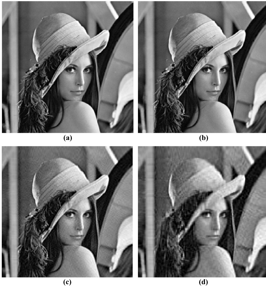
Fig. 1. (a) Original Lena image; Lena's image of size 256 \times 256 reconstructed by Eq. (4) using (b) 128 singular values, (c) 64 singular values and (d) 32 singular values.
