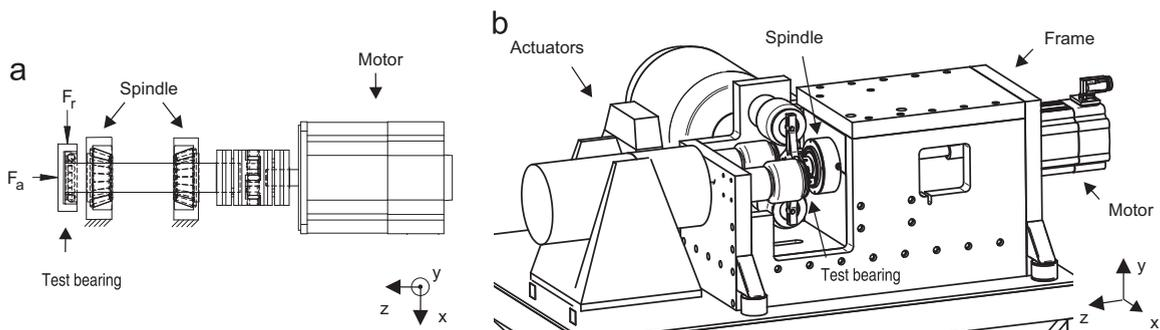
**Fig. 1.** Concept (a) and overview (b) of the presented test rig. The test bearing is mounted on a spindle and driven by an electric motor. The actuators apply a radial force ( $F_r$ ) and an axial force ( $F_a$ ) on the test bearing.
