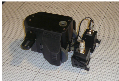
Fig. 1. RSA with air-coupled ultrasonic transducers attached. For a detailed description of the system architecture see [12]. Ultrasonic, magnetic flux leakage and eddy current sensors may be attached to the chassis in order to test the structure under investigation. Magnetic wheels are used to allow the robot to adhere to and negotiate 3D ferromagnetic structures.
