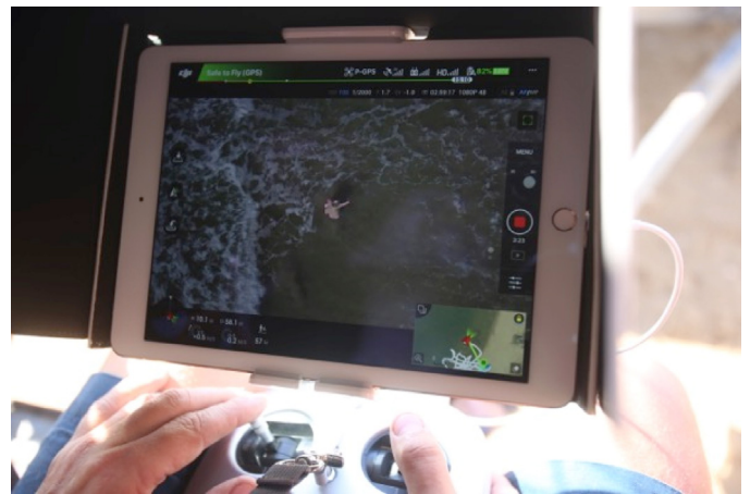
Fig. 2. UAV remote controller with tablet display iPad air 9,7".
