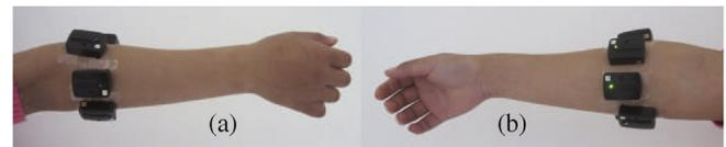
**Fig. 1.** Placement of EMG sensors: (a) posterior view; and (b) anterior view. Six wireless sensors were equidistantly placed around circumference of forearm in direction parallel to muscle fiber. Each sensor detected sEMG by a bipolar electrode.
