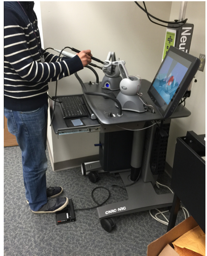
Fig. 1. NeuroTouch and User. The user is holding the endoscope in the left hand and the drill in the right hand. Pedals are positioned. The endoscopic view is demonstrated on an adjustable screen.
