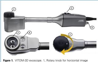
Figure 1. VITOM-3D exoscope. 1, Rotary knob for horizontal image adjustment. 2, Rocker switch to scroll in the menu/functions and control button to open menu/functions. 3, Stereo lens. 4, Light outlet—integrated illumination unit. 5, Connection to fiberoptic light cable.
