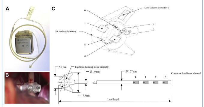
**Figure 1.** (**A**) Total implant system. The total implant system consists of the pulse generator, extension cable, and cuff electrode at the distal end of the electrode. In the latter cohort, an updated version of the pulse generator was used (Activa version [Medtronic]). (**B**) Implantation of the cuff electrode. The cuff electrode is placed around the cochleovestibular nerve,
