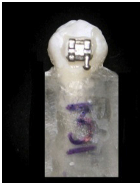
Fig 2. Mounted tooth in acrylic block after bonding.
