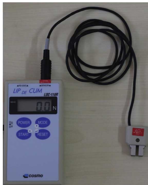
Fig. 1. Lip De Cum ® device (Cosmos instruments Co. Ltd, Tokyo, Japan) has two parts including a sensor with a lip adaptor and digital display.
