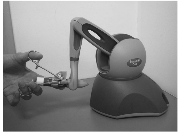
Fig. 1. Geomagic Touch. The Geomagic Touch device allows 3D spatial position (x, y, and z coordinates) and stylus pen direction (pitch, roll, and yaw) to be accurately measured. The device uses a motor to generate a force against the user's hand, allowing simulation of touch and interactions with virtual objects.
