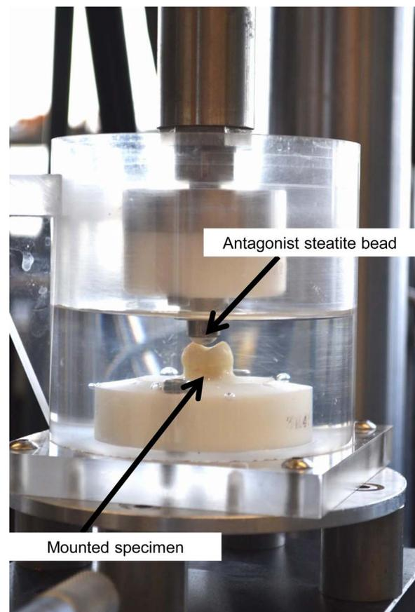
**Fig. 1.** Cyclic loading setup. Each tooth was mounted in acrylic resin and located in the lower chamber of the artificial oral environment. A steatite bead attached to the upper loading arm acted as the antagonist.
