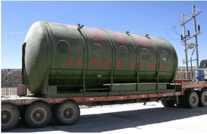
Fig. 1. The new multiplace plateau hyperbaric chamber (1 = Compressor; 2 = Doors; 3 = Control device; 4 = Desk; 5 = Beds; 6 = Gas vent; 7 = Air evacuation valve; 8 = Windows; 9 = Main compartment; 10 = Buffer compartment; 11 = Intake-tube; 12 = Silencer). Minimum pressure of the main compartment can reach up to 0.029 MPa at 355 m, 0.022 MPa at 2880 m and 0.02 MPa at 4532 m.
