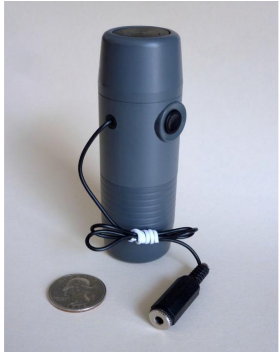
Fig. 1. A TruTone® EL modified to receive an input sine wave determining the instantaneous fundamental frequency ( F_0 ) of the EL voice. Quarter provides size reference.
