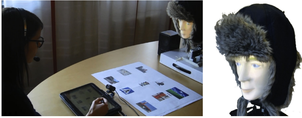
Fig. 1. The human–robot Map Task setup used in the study (left) and a close-up of the robot head Furhat (right).
