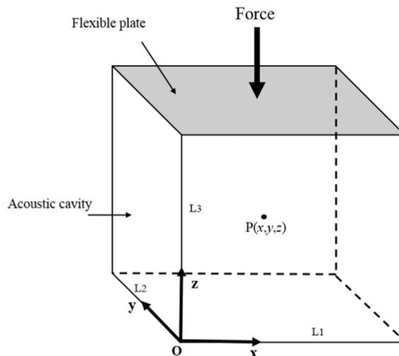
Fig. 1. A flexible plate-acoustic cavity system.
