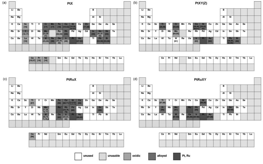
Fig. 1. Overview over the existing elemental compositions of DMFC anode catalysts of (a) PtX, (b) PtXY(Z), (c) PtRuX and (d) PtRuXY. Elements are labelled whether reported as oxidic phase or alloyed with the Pt, Ru; unused and unusable. Associated literature is referenced [16–27,29,30–52,54–57,60–65,67,68,70,72–78,80,81–86,88,89,92–94,96].
