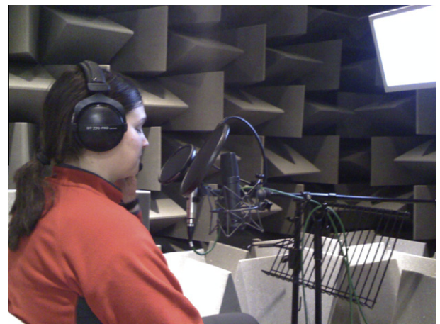
Fig. 1. Studio setup for recordings. Left microphone is a Sennheiser MKH 800 and the right one is a Neumann u89i. The headset has a DPA 4035 microphone mounted on it.
