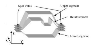
Fig. 2. Thin-walled cross section of BIW structure using pressed sheet metal.
