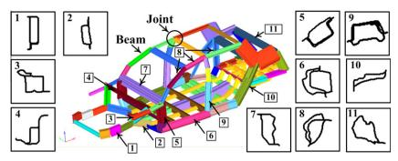
Fig. 1. BIW frame structure and its thin-walled cross section.
