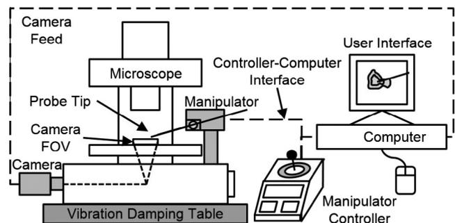
**Fig. 2.** System layout illustrating the transfer of information between system components. The camera observing the microscope slide is directly connected to the computer, which is in turn connected to the manipulator controller. The manipulator controller processes either signals from the computer or the manual input device depending on which method of control is enabled.
