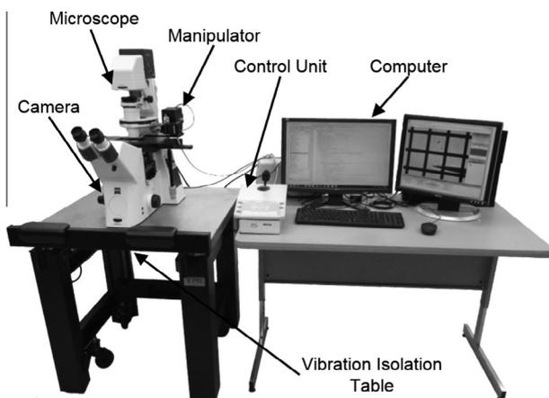
**Fig. 1.** System layout used in the development of the nanomanipulator GUI. The layout consists of a microscope, camera, manipulator with control unit, and a standard computer workstation containing the Manipulator Control software.
