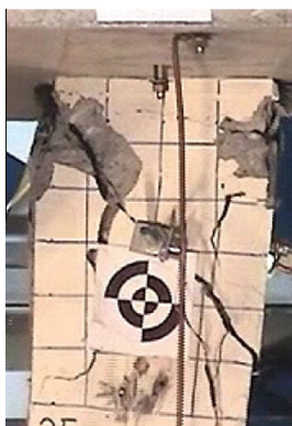
Fig. 1b. A 45-degree crack indicating shear failure.
