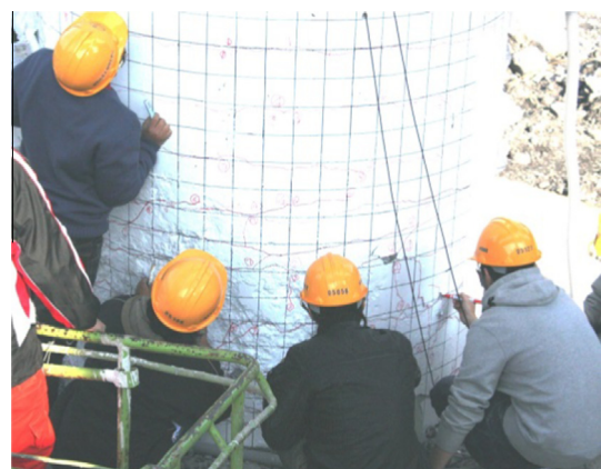
Fig. 2. Manual pen marking on cracks.
