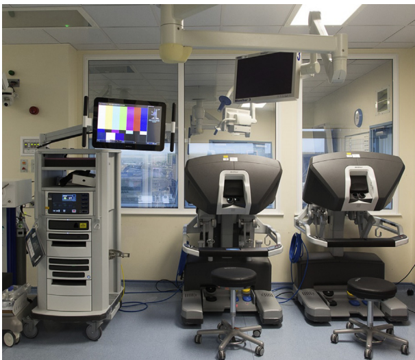
Figure 2 On the right; dual surgeon console. On the left; vision cart. The second surgeon console is for training purposes.
