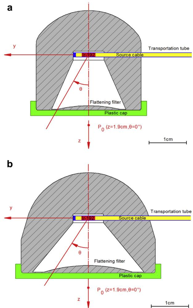
Fig. 1. The geometrical design of the Bebig (a) BVH-20 and (b) BVH-30 skin applicators with their corresponding flattening filters provided by the manufacturer. The coordinate origin depicts the position of the source center inside both skin applicators, and the point  $P_0$  is the reference point in water along the z-axis of symmetry ( $y = 0 \text{ cm}$ ) in the depth of  $d = 0.3 \text{ cm}$  ( $z = 1.9 \text{ cm}$ ). Ir-192 = iridium-192.
