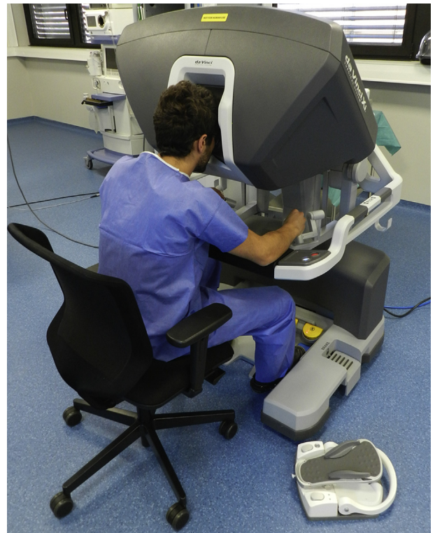
Figure 1. Remote console of the robotic surgical system. The surgeon's console is equipped with an optical viewing system, 2 telemanipulation handles, and 5 pedals. The optical viewing system, called the stereo viewer, provides a 3-D view of the operating field. The 2 handles allow remote manipulation of the articulated robotic arms. The phaco handpiece is controlled with the pedal installed next to the robot's pedals.
