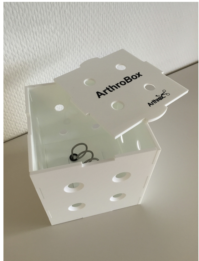
Fig 1. The arthroscopic training device is depicted and shown with the top-piece moved aside to have a good view in the inside showing the skill plug with the metallic helix and rubber ring.
