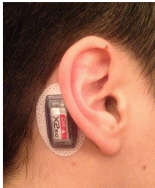
Fig. 2. X2 Biosystems xPatch sensor applied to an athlete. The application area was prepped with 3M Cavilon No Sting Barrier Film Spray (3M Health Care, St. Paul, MN). The sensor was then turned on using the X2Biosystems case and applied to the adhesive patch. The patch was then applied behind the right ear of the athlete with the arrow on the sensor pointing towards the ear.
