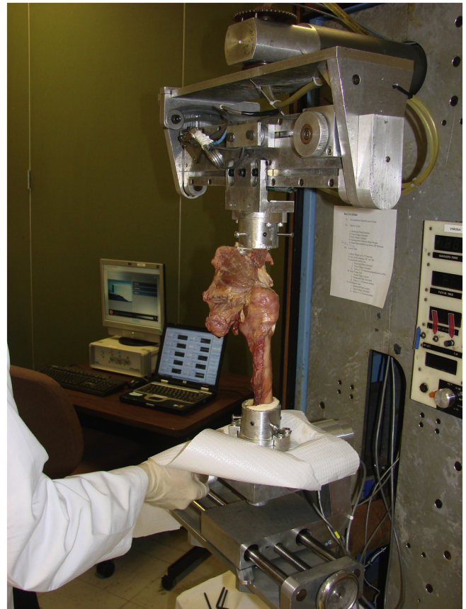
Fig. 1. Anatomic hip specimen in the joint simulator being tested in 0° of extension.
