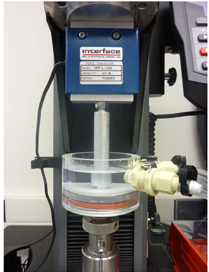
Fig. 1. Experimental setup for unconfined compression tests. Fibrin gels were submerged in a PBS bath maintained at 37 °C.
