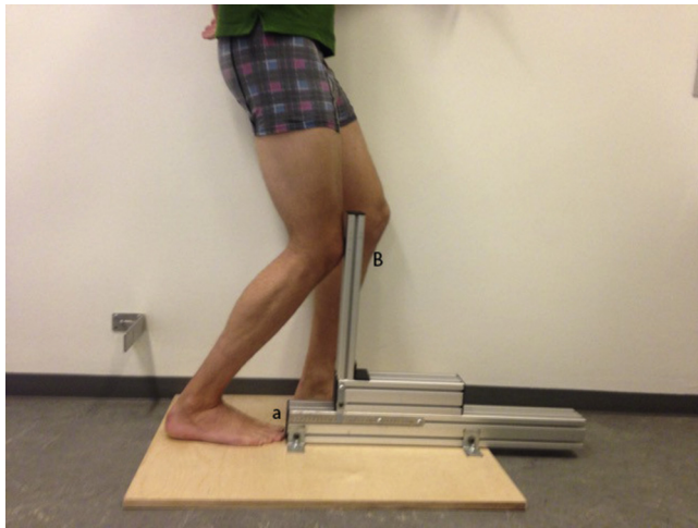
Fig. 1. The test procedure, showing the (a) fixed datum adjacent the toe and (b) the measurement indicator at the anterior knee.
