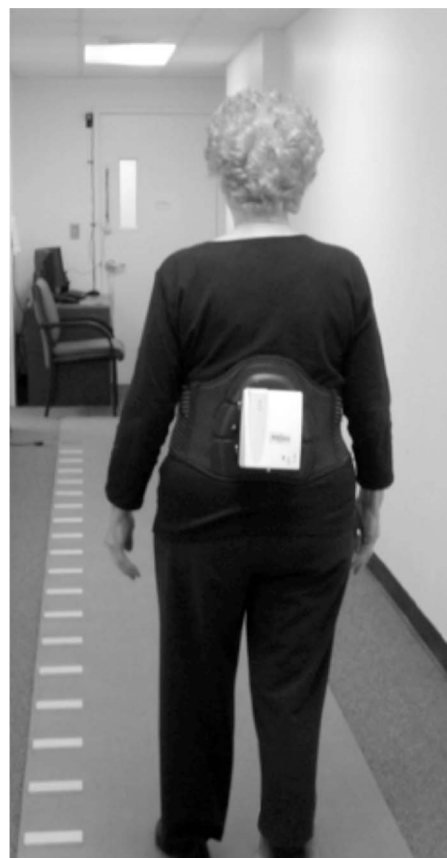
Fig. 1. Depicts a CCMA participant with the wireless Swaystar device system fastened around their lower back.
