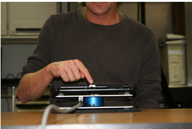
Fig. 1. Experimental set-up. Participants were seated with the touchscreen tablet centered on a table in front of them. The tablet was affixed rigidly to a force transducer that measured the forces applied on the touchscreen.
