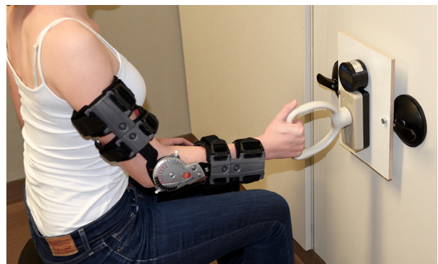
Figure 2 Forearm supination strength measurement. The participant was seated with shoulder and elbow in approximately 45° of flexion, grasping the T-handle with the forearm in neutral position.
