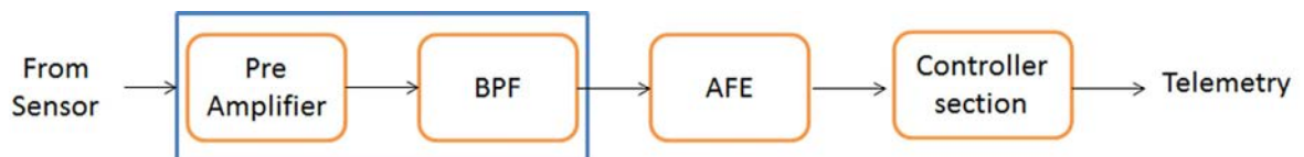
Fig 1: Block diagram of front end receiver of an underwater imaging sonar
