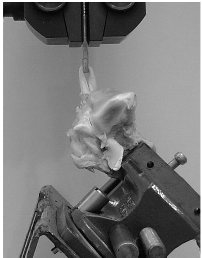
Figure 2. Tibia specimen prepared for the test. The loop of tendon placed on the upper part is observed.
