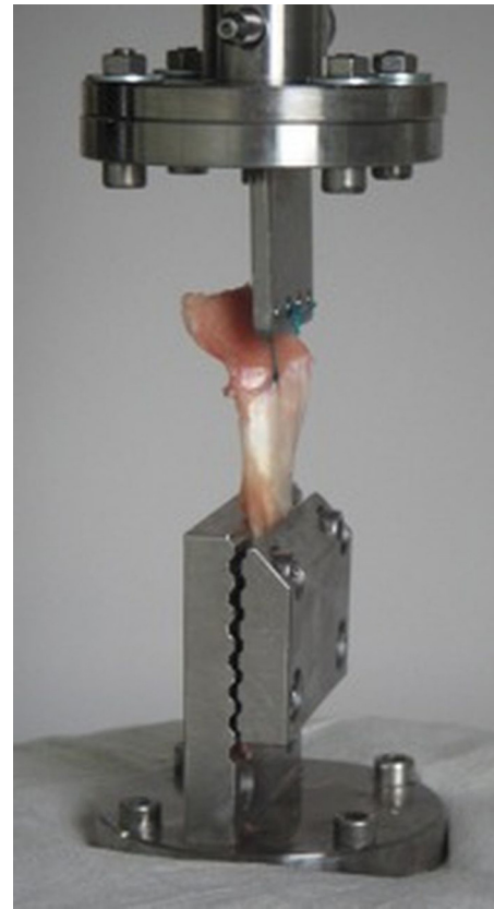
Fig. 1. Experimental set-up with fin-like design at the upper support and a clamp at the bottom base, with suture refixation.
