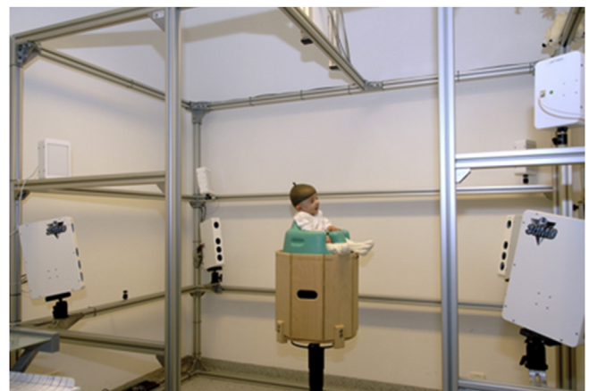
Fig. 1. Acquisition of a 3D stereophotogrammetry of a dummy. The infant is placed in the center of five synchronized camera pods. Image acquisition takes less than 1.5 ms, meaning that it is free of movement artifacts.
