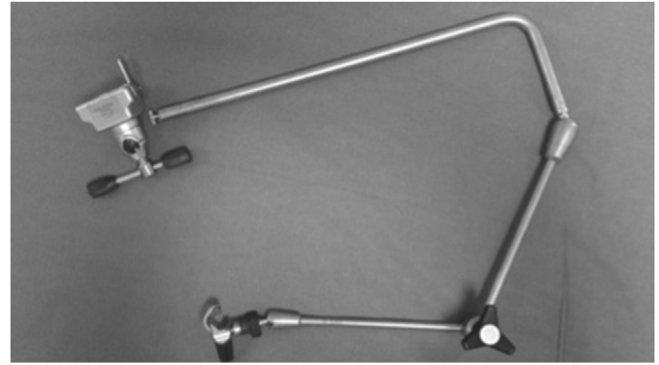
Fig. 3. Mechanical articulated holder.
