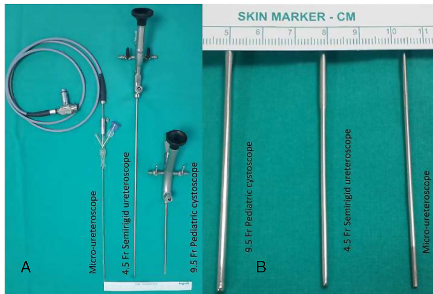
Fig. 1. The micro-ureteroscope, 4.5Fr semirigid ureteroscope and 9.5Fr pediatric cystoscope are set ready on the operating table.
