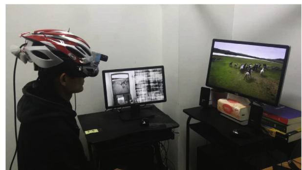
Fig. 1. The alter reality system and an example of the experimental scene. The system comprised of a camera connected to a computer that fed into the HMD. This computer processed the images taken by the camera in real-time, and then presented the images to the HMD. The original image was presented to one eye, while the altered image to the other eye. Participants wore the HMD during adaptation when they could view the world freely or watch movies as shown in the figure. The small LCD monitor was also connected to the computer, which worked in a clone mode with the HMD. This enabled the experimenters to see what the subject viewed. In this example, the subject was watching the original camera video through the left eye, and the pink noise video through the right eye.
