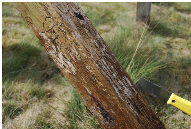
Fig. 1. Evidence of decay on the in-ground portion of a WRC fence post after 6 years in Maple Ridge, British Columbia.
