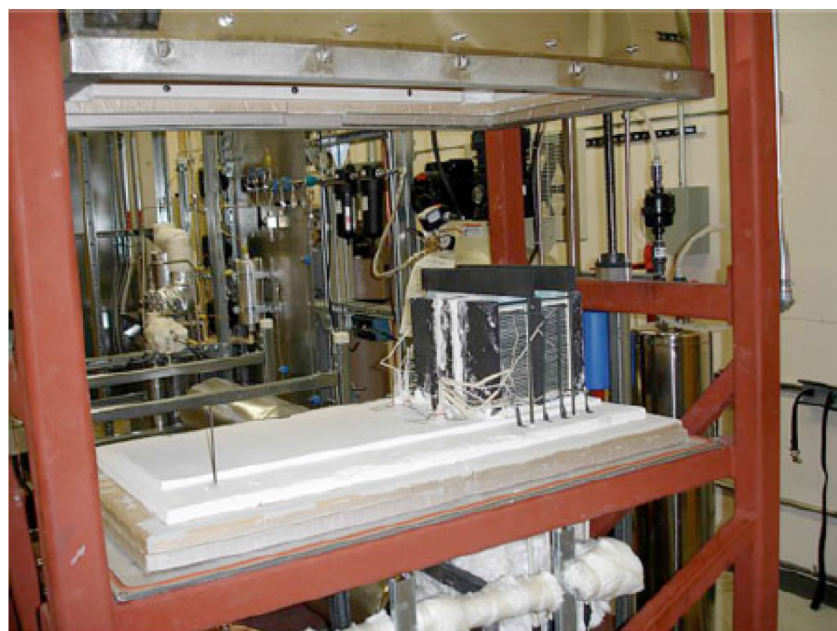
Figure 2. The large furnace with one electrolysis stack in place.
