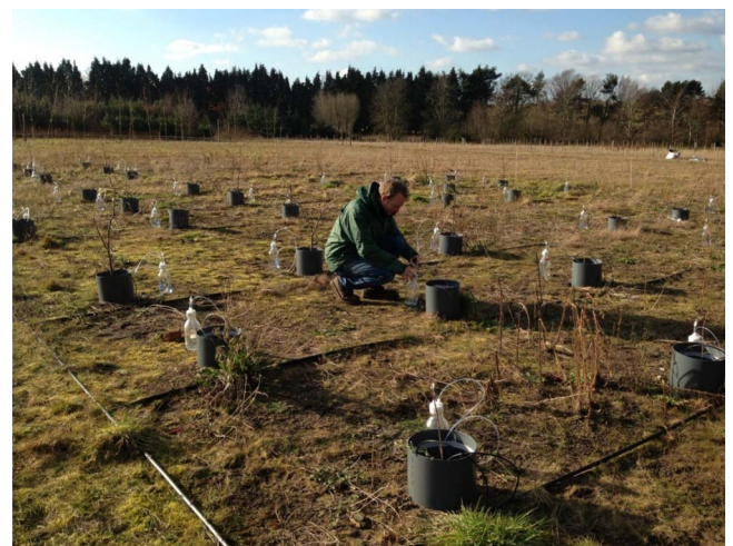
Fig. 2. Inspection of mesocosms. In the foreground the drip-irrigation system is visible, as are the white velcro strips within the experimental tubes to prevent earthworm escape.
