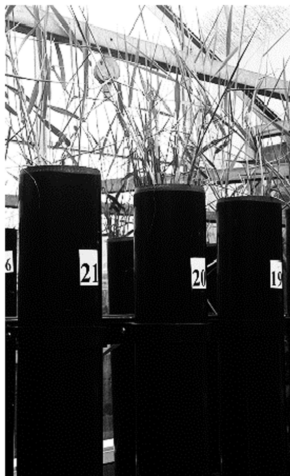
Fig. 1. Experimental vertical-flow constructed wetland rig located within a greenhouse at the beginning of the experiment (Picture taken by Mr. Amjad Hussein on 15 May 2015).
